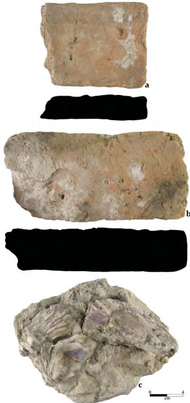
Figure 3-57. Structural materials: (a-b) French-style bricks with drawn profiles (Area 3, FS 1018); (c) tabby mortar with oyster shells (Area 6, FS 980).
