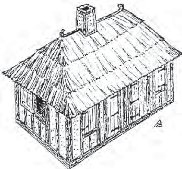
Figure 6-3. Drawing of a poteaux sur sole structure at Old Mobile (by Philippe Oszuscik).
